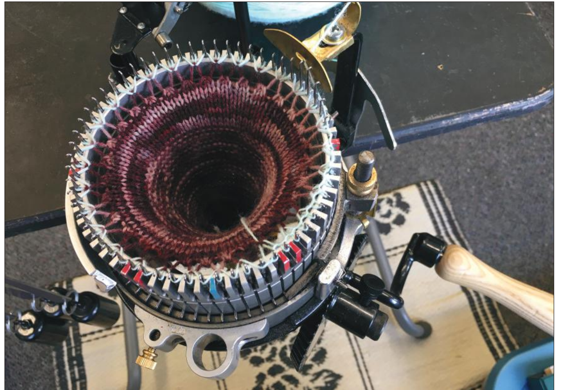
A CLOSE-UP VIEW of the antique sock machine demonstrated last weekend at the Brandon Library by Bonny Dutton. The intricate, diabolically clever mechanism initially required careful counting in order to ensure the proper number of turns. A digital device now keeps track.
